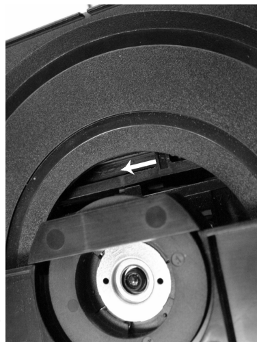
Manually opening of tray When it is not possible to open the tray with the EJECT button, the tray can manually be opened. When no disc is loaded, unlock the tray by moving the slide from left to right and pull tray outwards.
